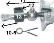
15. Lay spring over finger of adaptor and line up hole in aluminum housing
