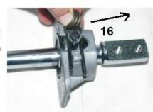
16. Twis spring upward twards top of adaptor.
